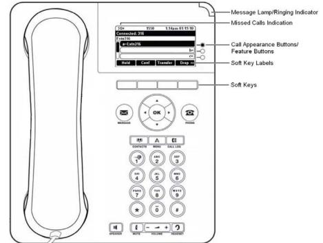
The phone supports 12 programmable call appearance/feature buttons. The labels for 3 of these are displayed in the main display and can be controlled by the adjacent buttons to the right. You can use the  $\blacktriangle$  up and down  $\forall$  arrow keys to scroll the display. You can also use the  $\blacktriangleleft$  left and right  $\blacktriangleright$  arrow keys to move through the button feature in pages of 3.
