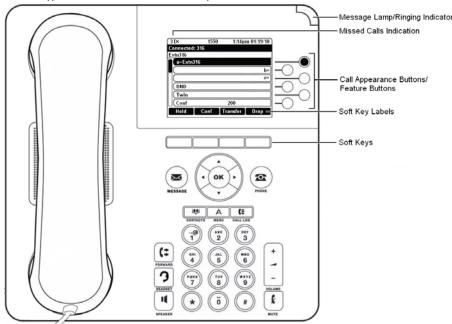
The phone supports 24 programmable call appearance/feature buttons. The labels for 6 of these are displayed in the main display and can be controlled by the adjacent buttons to the right. You can use the  $\triangle$  up and down  $\nabla$  arrow keys to scroll the display. You can also use the  $\triangleleft$  left and right  $\triangleright$  arrow keys to move through the button feature in pages of 6.
